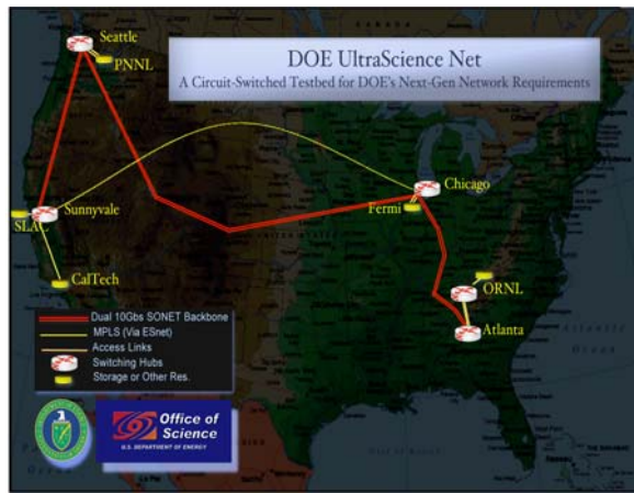
Figure 1. USN showing the span provided by dual 20 Gbs lambdas.
