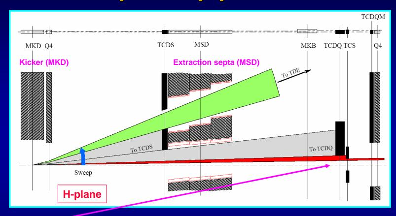
The <u>TCDQ absorber</u> downstream of the dump kickers will be positioned to protect machine elements / apertures from the dump sweep. The TCDQ will be positioned at to shadow the apertures (not the collimators !)  $\rightarrow$  distance of  $\approx$ 8-10 $\sigma$  during most operational phases.
