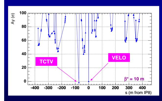
The plot shows the ~ aperture with the orbit bump around IR8 (in r.m.s. beam size).
