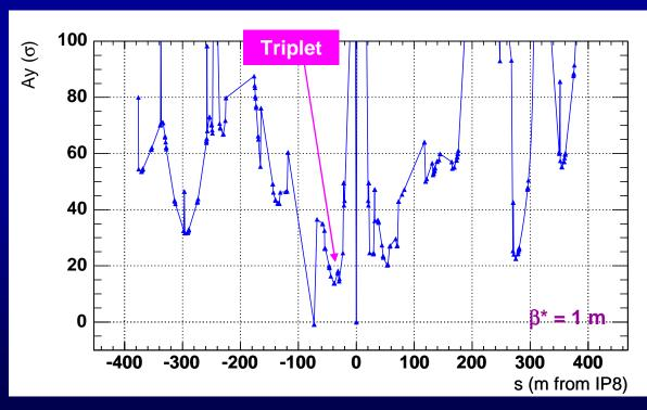
Note that for this aperture evaluation, only a misalignment of 2 mm has been taken into account. In reality the triplet apertures may be smaller, but not sufficiently to protect VELO.
