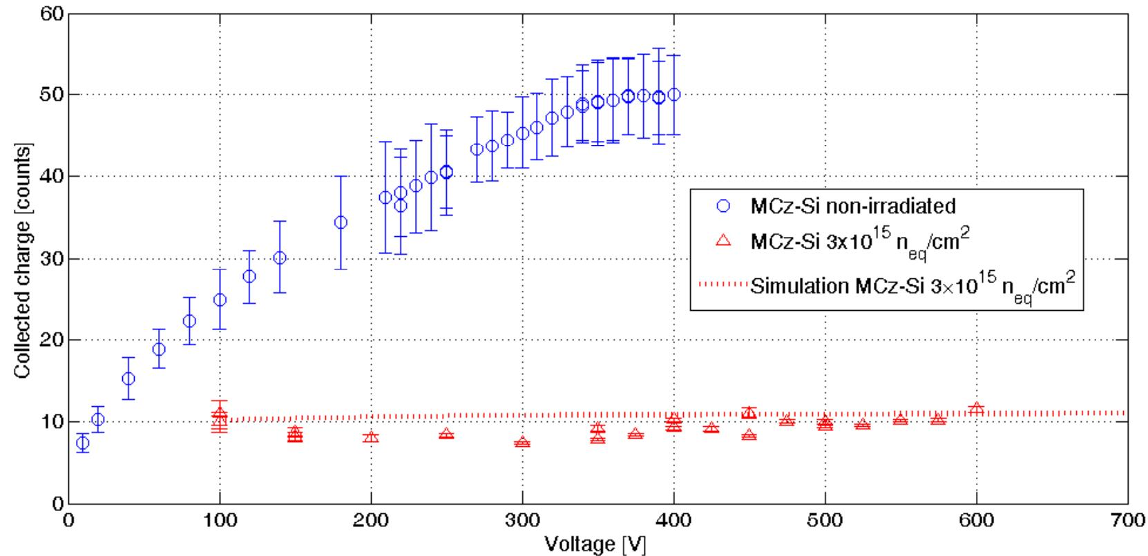
➤ The signal of the MCz detector irradiated to the fluence of  $3 \times 10^{15}$  1 MeV  $n_{eq}/cm^2$  is approximately 20% compared to the non-irradiated device.
