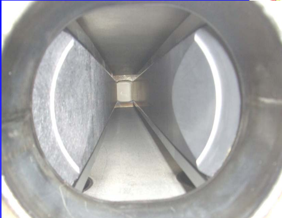
C-C (left) and C (right) jaws after impact
