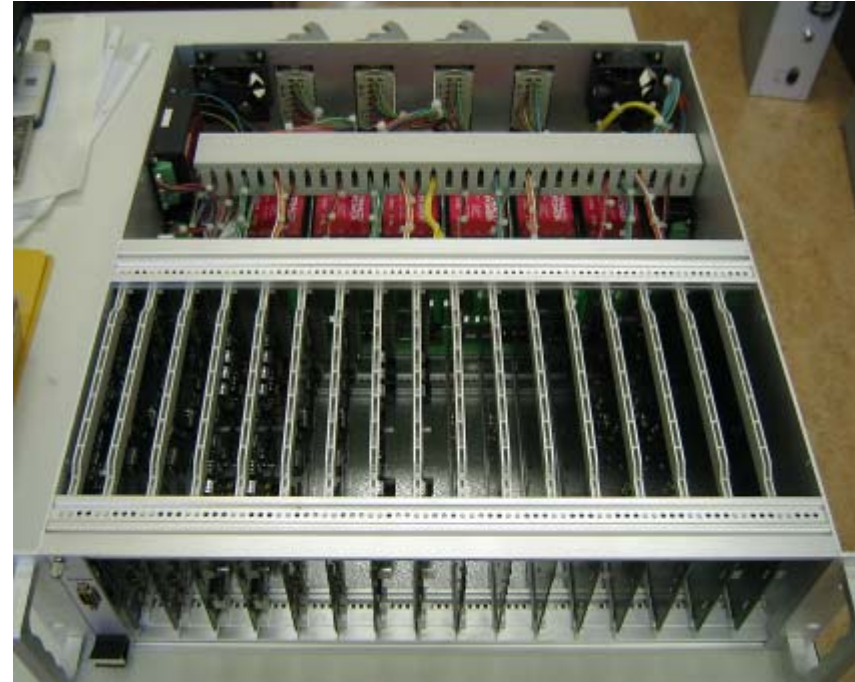
Type A Global Protection Unit for up to 4 corrector magnet circuits. The unit is attached to dedicated 600 A current sensors.
