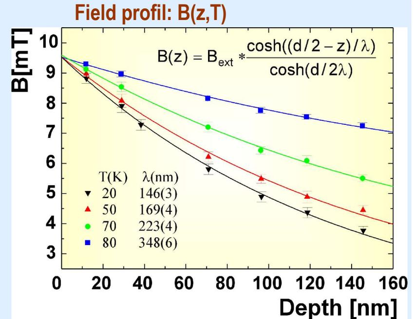
With very low energy muons we probe nanometer thick magnetic layers
