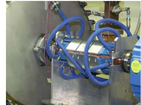
RF deflectors (INFN-LNF)
