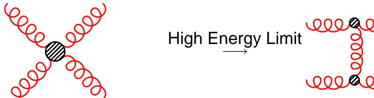
Diagrams with a t-channel gluon exchange dominate the cross section.
