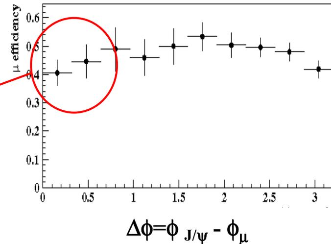
Contrary to CDF run-I measurements with  $b$ -jet +  $\mu$ , use of excl. B channels allows high efficiency also at  $\Delta\phi \rightarrow 0$
