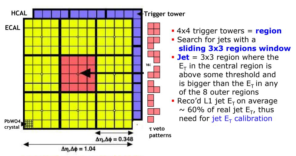
A jet = 144 trigger towers, with typical tower dimensions  $\Delta \eta \times \Delta \phi = 0.09 \times 0.09$ Hence typical jet dimensions:  $\Delta \eta \times \Delta \phi = 1 \times 1$
