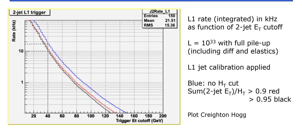
Possible L1 condition that comes closest to a rap gap trigger (rap gap > 2): **2 jets in central Cal (|\eta|<<b>3)with**  $\Sigma(E_T 2 \text{ jets}) / H_T > \text{threshold}$  $H_T = \text{sum of the scalar } E_T \text{ of all jets in the event with } E_T(jet) > \text{threshold}$
