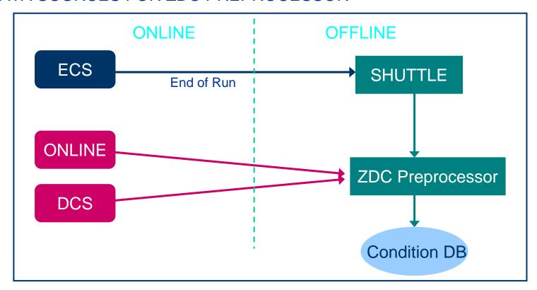
Output of ZDC online calibration routines ⇒ input data for Shuttle
