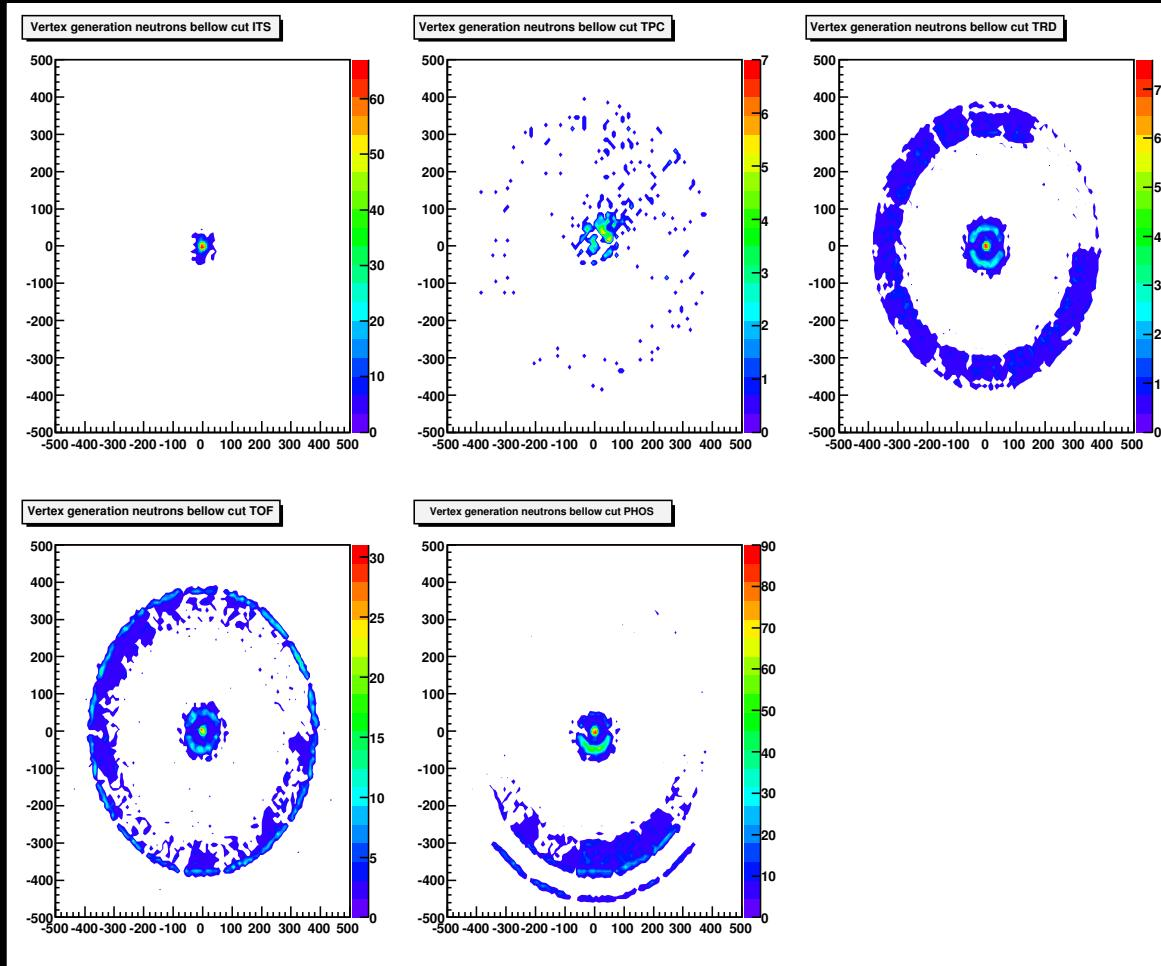
Vertex creation of  $\gamma$  from forced capture in GEANT3 for 100 keV cut off
