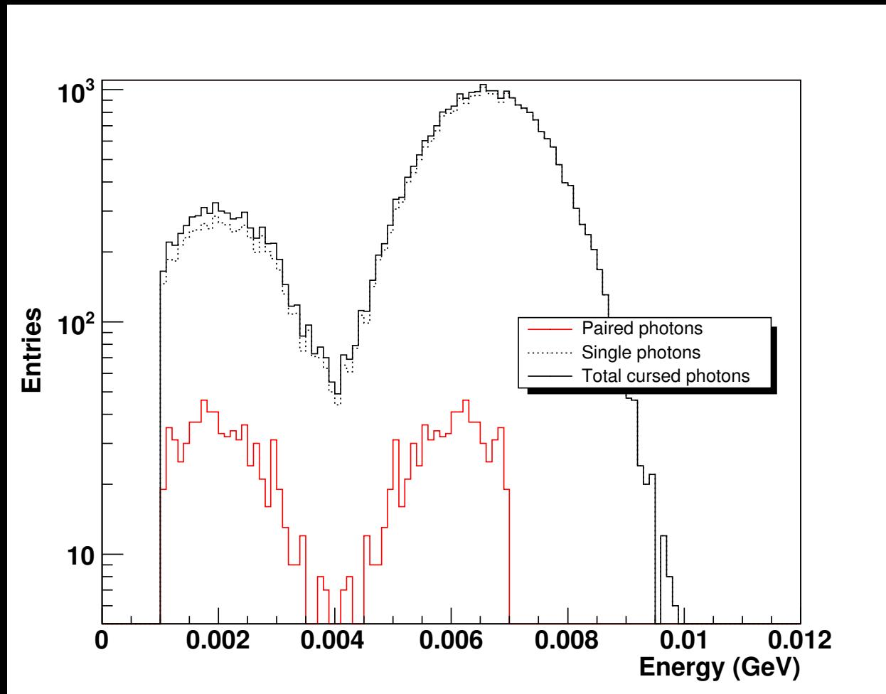
Correlation of photon spectrum due forced capture to parent neutron kinetic energy in GEANT3 for 1 MeV cut off.
