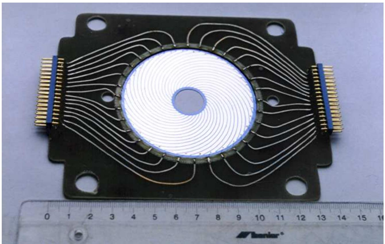
Measurements of light charged particles ( $p, d, t, \alpha, {}^6\text{Li}$ ) produced in the  ${}^{14}\text{N}({}^{12}\text{C}, X)$  reaction by E- $\Delta E$  telescope consisting of 52  $\mu\text{m}$  thick  $\Delta E$  strip detector followed by Si(Li) E detector.
