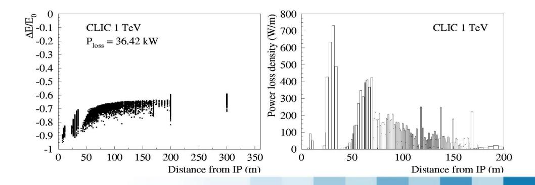
Beam losses in the 20 mrad extraction line of a TeV linear collider:
