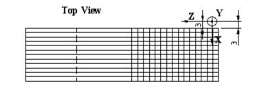
Initial design uses 2 mm<sup>2</sup> rods, gives x segmentation: could help with multiple proton events (enough light?)
