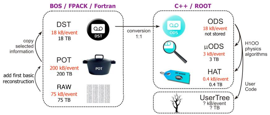
We don't want to re-write all the reconstruction software, instead: a 1:1 conversion from DST to ODS: H1Track, H1Cluster objects generic reading of BOS banks
