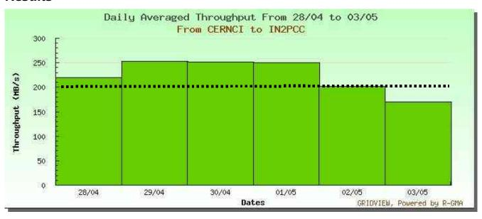
It was proved that IN2P3 could sustain nominal rate and above (+25%) for a few days using the same infrastructure as first period. Adding the 4<sup>th</sup> server allowed to run 25% more than the nominal rate. It was switched off on early 02/05 and the nominal rate was sustained that day despite a CASTOR problem in the afternoon (see SC4 blog).
