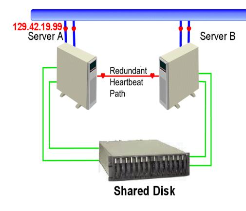
Redundancy eliminates Single Points Of Failure (SPOF)
