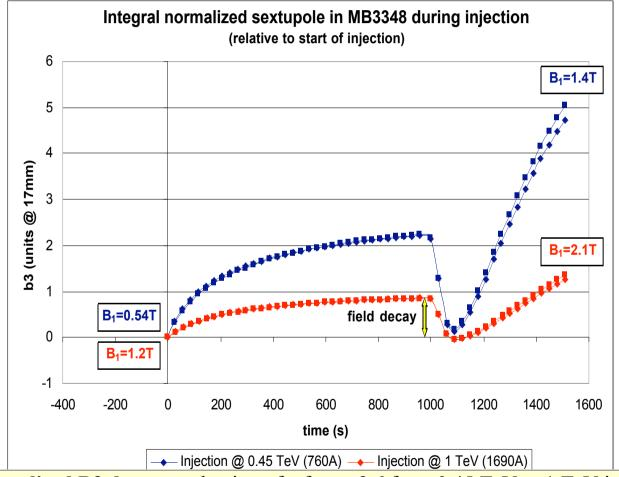
Normalized B3 decay: reduction of a factor 2.6 from 0.45 TeV to 1 TeV injection
