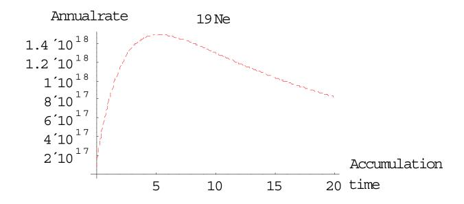
The annual neutrino rate as a function of the accumulation time in the EC-RCS and stacked in **PS** at 10 Hz injection.
