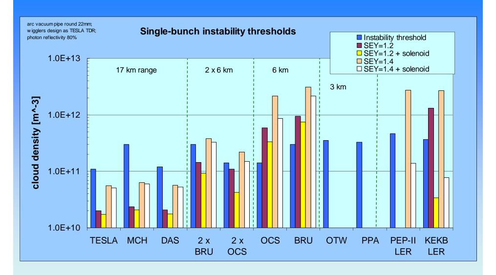
Single bunch instability threshold and simulated electron cloud build-up density values for a peak SEY=1.2 and 1.4.
