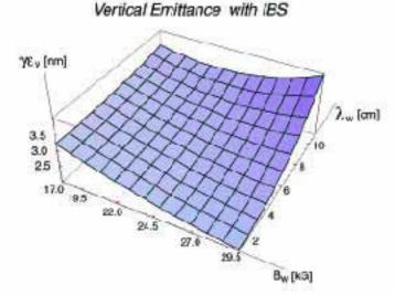
$\gamma \varepsilon_x = 400 \text{ nm}$   $\gamma \varepsilon_z = 2 \text{ nm}$  at 2.4 GeV incl. IBS
