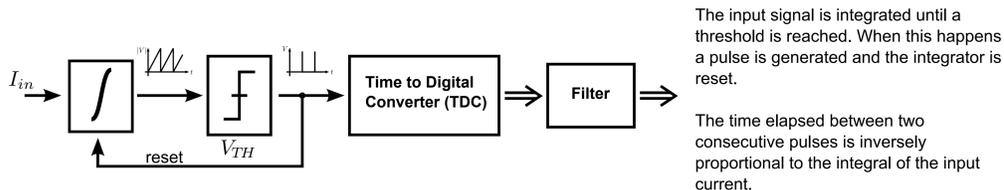
The input signal is integrated until a threshold is reached. When this happens a pulse is generated and the integrator is reset.
