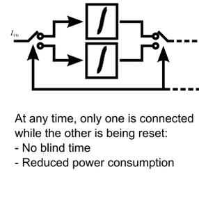
At any time, only one is connected while the other is being reset:
