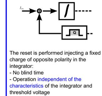
The reset is performed injecting a fixed charge of opposite polarity in the integrator:
