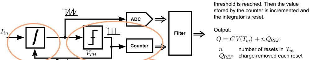
The input signal is integrated until a threshold is reached. Then the value stored by the counter is incremented and the integrator is reset.
