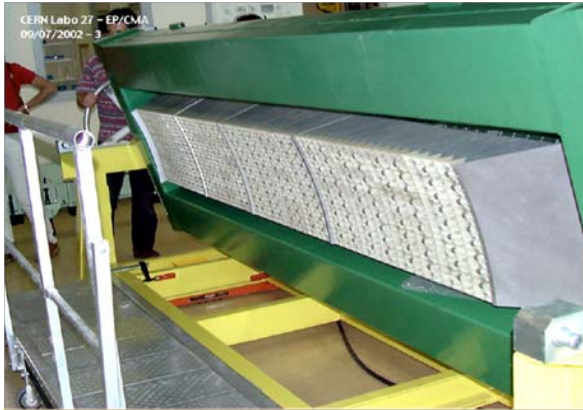
A CMS Supermodule with 1700 tungstate crystals
