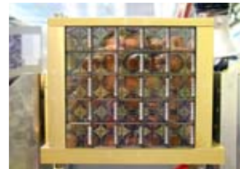
A CMS endcap 'supercrystal' 25 crystals/VPTs
