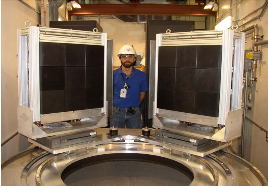
Anger camera with GS20 scintillators, developed at SNS for Crystallography instruments
