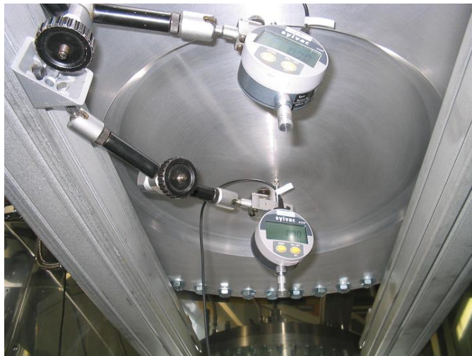
Pressure test (0 to 21.5 bar)
