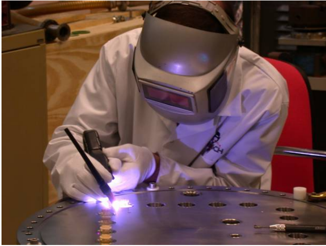
TIG welding of 20 HV 37pts feedthroughs connectors and gas feedthroughs
