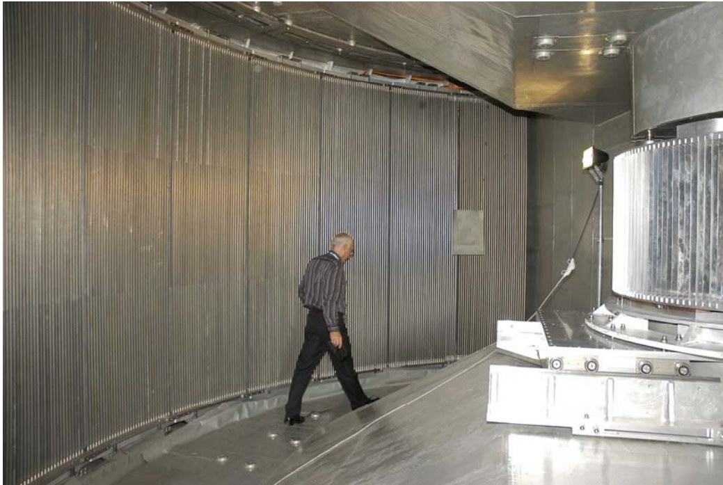
The 30 m 2 detector of the IN5 Energy spectrometer at the ILL
