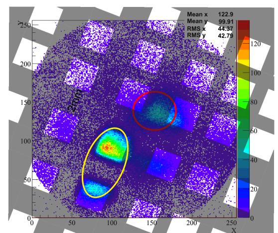
Gaussian fit:  $\sigma_r = 365.8 \mu m$  $\sigma_{l} = 362.1 \ \mu m$  $\sigma_{\text{optics}} = 300 \ \mu \text{m}$
