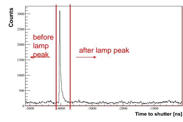
Ion feedback produces clusters of pixels in one time bin → identification to reduce the dark rate
