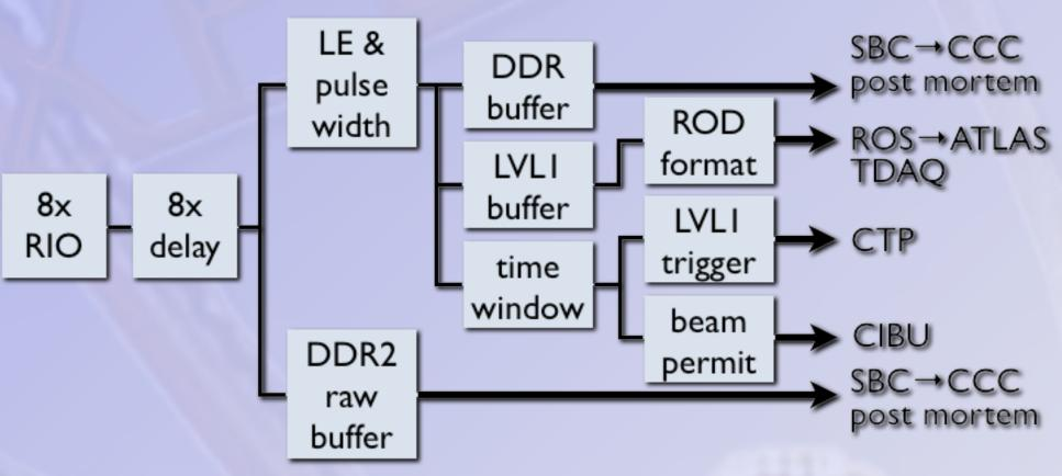
A Level1 buffer stores the processed data together with a bunch crossing identifier. Input Trigger signals are used to select data which are fed via a optical gigabit link to the Read Out Subsystem (ROS) and the subsequent standard ATLAS DAQ readout chain.
