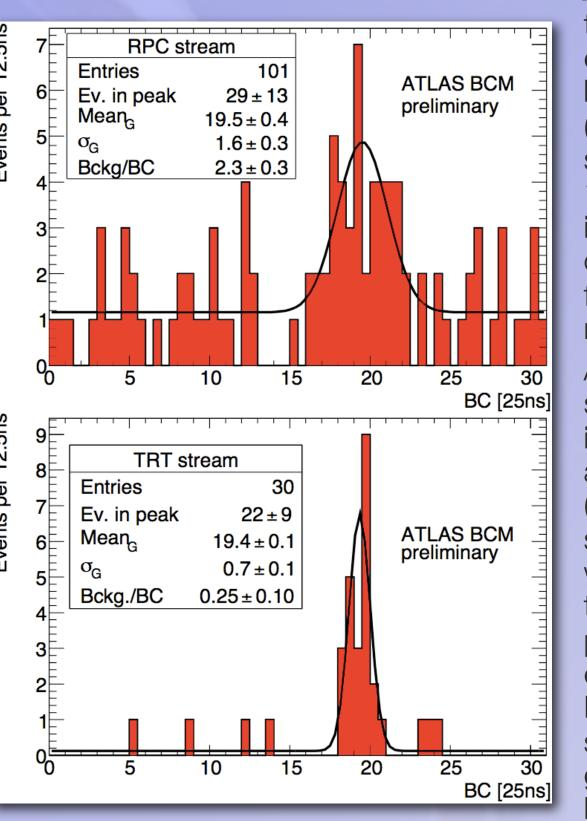
For each trigger from the CTP the BCM reads out 31 consecutive bunch crossings (LVL1As). Most hits showed up in LVL1A bin 19 as expected from an initial timing calibration on the basis of cable and fiber length measurements.
