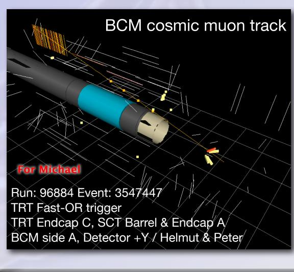
in the TRT triggered data stream. Examples for cosmic muon tracks through BCM detectors are shown for each of the triggers with hits in the TRT and SCT barrels and endcaps.
