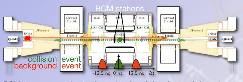
BCM detectors need to be fast with signal rise times of about 1 ns, pulse widths around 3 ns and baseline restoration times in the order of 10 ns. Close to the beampipe they have to withstand radiation doses up to 50 MRad during the 10 years
