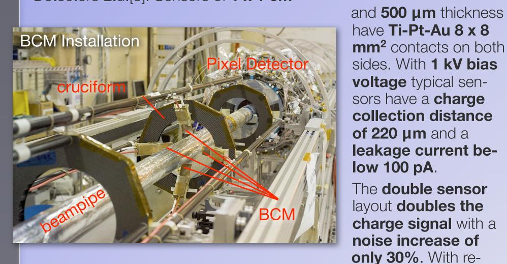
spect to the beam axis the sensors are mounted tilted at 45°. With a most probable MIP energy loss of 9.0 ke<sup>-</sup> (mean: 11.3 ke<sup>-</sup>) signal/noise ratios of ~10 are achieved.
