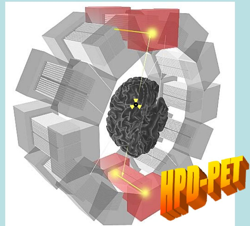
Arrays of long ( $L_c \sim 10\text{--}20\text{ cm}$ ) crystal bars
