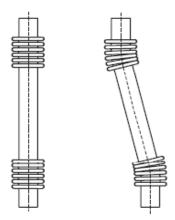
Besides economical advantages, the use of an intermediate tube increases the resistance to internal pressure and the total number of corrugations is lower than in a "continuous" bellows and the corresponding reduction factor  $k_i$  (see page 63) will increase (come closer to 1).
