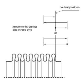
The pressures and movements quoted in the data sheets have thus been specified that in the case of cold stress (room temperature 20–30 °C) and expert installation at least
