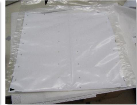
Reflector foil before/after TPB evaporation
