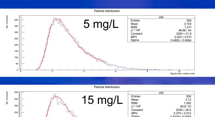
Adding MSB to the PC+PPO sample decreases the light yield as seen by PMTs. As more is added, the less light is detected.
