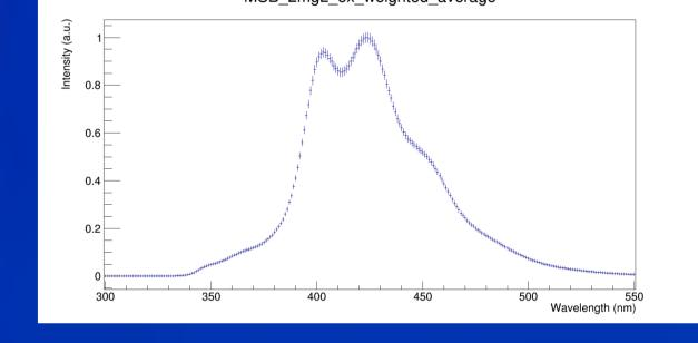
To understand the contribution of MSB, its spectrum was also recorded as exited by ~380nm light range. No light emitted MSB exciting by 275 nm, so only contribution from PPO was included in the process.
