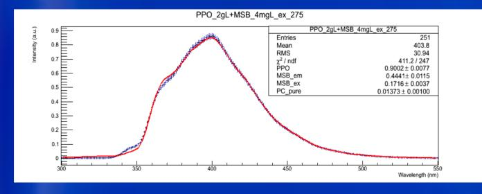
To see what happens: spectra for several different concentrations of MSB in the sample were observed. All the spectra of components were averaged and then used to make a fit of the light emitted by the sample.
