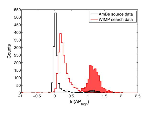
The anomalous background is overlapping with nuclear recoil data in acoustic power
