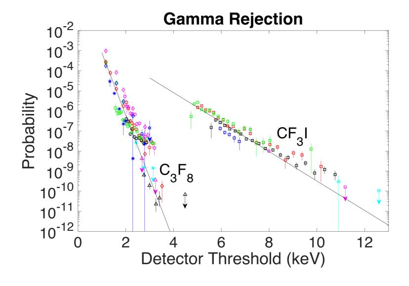
Probability of detecting gamma interactions in CF<sub>3</sub>I and in C<sub>3</sub>F<sub>8</sub>
