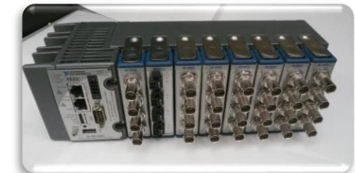
*Data acquisition system CompactRIO by NI 40 MHz*
