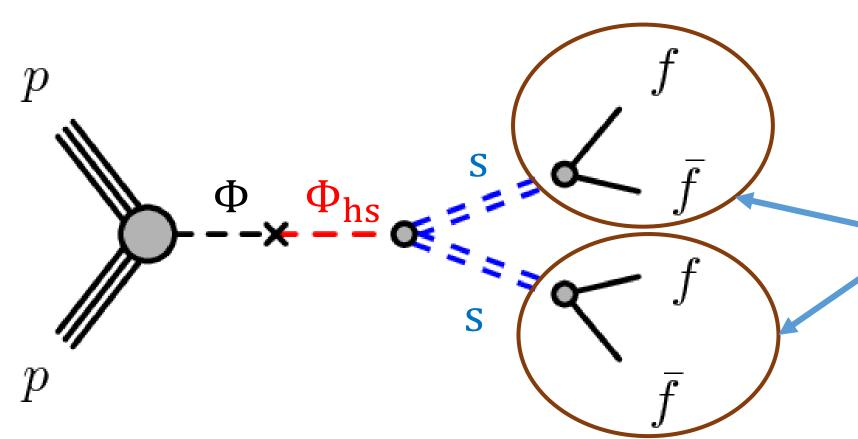
Topology is 4 heavy fermions, almost always b quarks, appearing somewhere in the detector. Depending on kinematics and the detector where they appear, the  $f\bar{f}$  pair won't always be resolvable as individual objects.
