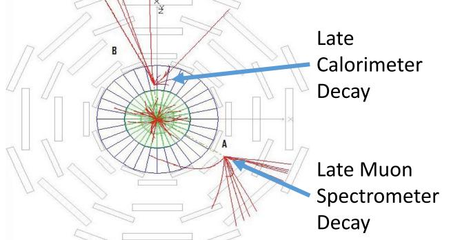
the jet axis. • A late decay in the EM calorimeter or in the hadronic calorimeter means a no or little energy deposited in the EM calorimeter. We use a requirement on the log of the CalRatio variable,
