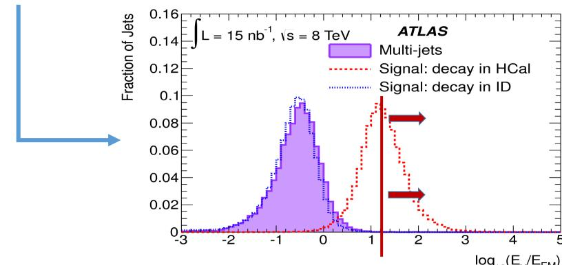
$\leftarrow$  The probability of detecting a s decay is a function of where it decays in the calorimeter.
