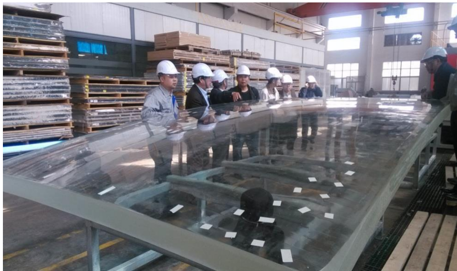
Forming panel size: 3m x 8m x120mm
