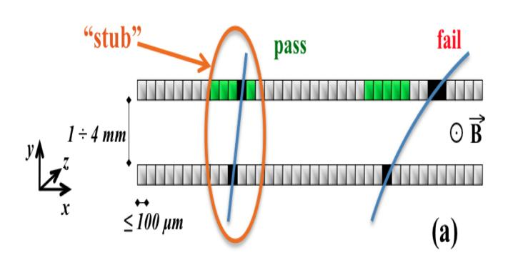
On-detector selective data readout - stubs: pair of correlated FE signals from a module ( $p_T$  > threshold (tunable)).
