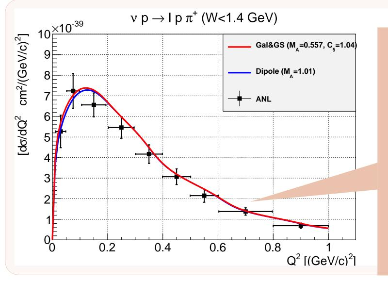
Flux-averaged differential cross-section  $d\sigma/dQ^2$  for  $p\pi^+$ final state with W < 1.4 GeVcut compared with ANL data. different curves show different sets of form-factors. RS and dipole versus Graczyk-Sobczyk and Galster for resonance and bkg models respectively after fitting the axial parameters
