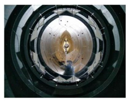
2.5 cm thick glass coated with Al Thin dielectric film added
