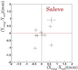
All mirrors aligned within 1 mm with respect to the reference
