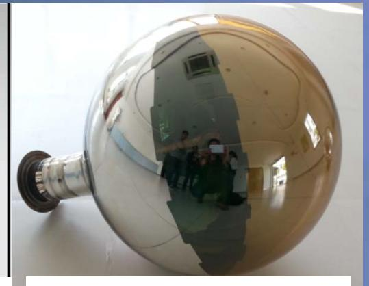
**Requirement:** High QE 20 inch PMT; Good SPE detection capability; Wide dynamic range; Low radioactive background; More than 20 years lifetime; Can withstand 0.4MPa Pressure; > 20000 pieces;
