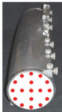
17 NMR trolley probes
