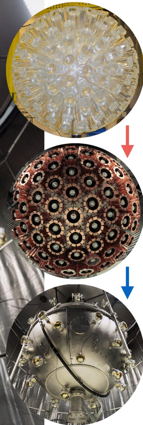
The contribution from Cherenkov activity in the acrylic, was considerably reduced as the water shielding tank was filled with ultra-purified Water.
