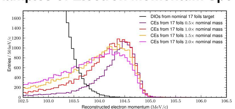
Examples of electron spectra of signal conversion electrons (CE) and decay-in-orbit (DIO) background electrons for stopping targets composed of 17 foils at different masses. The different signal shapes induced by multiple Coulomb scattering are apparent.
