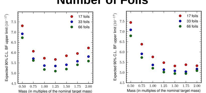
The optimization studies are performed with the expected upper limit on the conversion branching fraction as figure of merit. Overall, stopping targets composed of thinner and more foils perform better.
