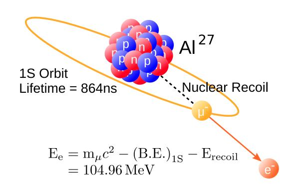
The conversion of muons to electrons in the field of an atomic nucleus is a coherent process and has the kinematics of a two-body decay. The conversion electron is mono-energetic with an energy slightly below the muon mass. Corrected for the nuclear recoil and the binding energy in aluminum, the experimental signature is a single 104.96 MeV electron.
