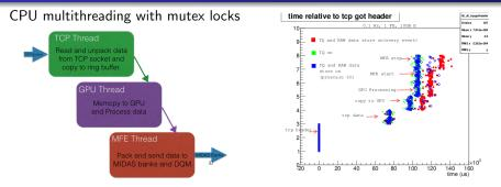
CUDA kernel routines: Data is copied to GPU memory in GPU thread, and then accessed by the following functions to identify and save islands, which are copied back to the computer memory and sent to the event builder.
