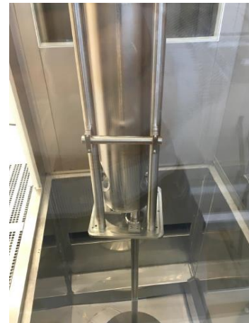
Prototype QWR für IBS RISP project in cleanroom, at high pressure water rinse (HPR) and 120 C bake
