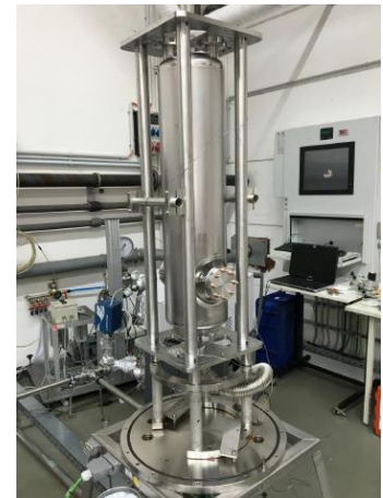
Prototype QWR für IBS RISP project in cleanroom, at high pressure water rinse (HPR) and 120 C bake
