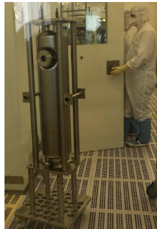
Prototype QWR für IBS RISP project in cleanroom, at high pressure water rinse (HPR) and 120 C bake
