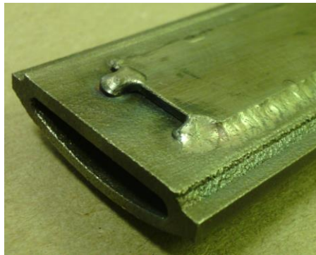
3D printed cooling channel
