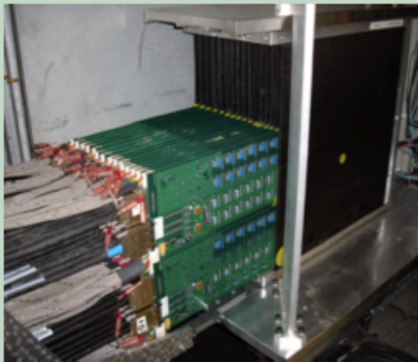
Si-W ECAL: 30 layers, 1 \times 1 \text{ cm}^2 cells
