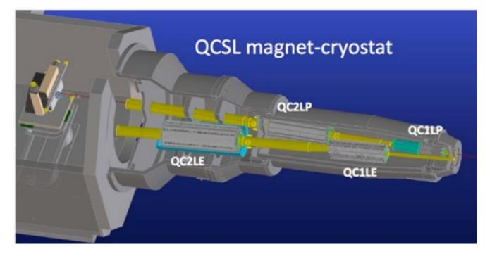
4 quadrupoles (QC1, QC2) + 16 corrector coils + 4 cancel coils (for leakage field) + anti-solenoid for the left side
