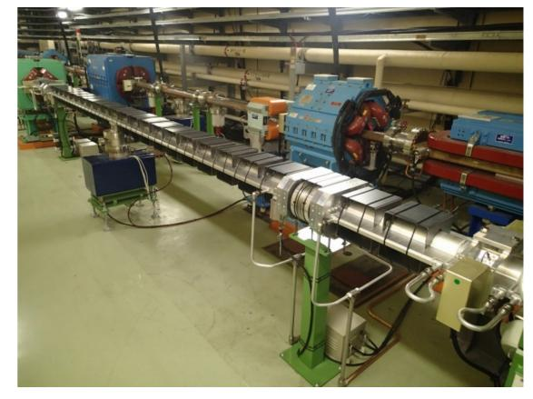
Ante-chamber and TiN coating is not enough to suppress EC at higher than 1 [A] beam current.
