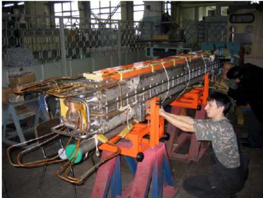
Figure 17 SIS100 curved magnet assembled without vacuum chamber.
