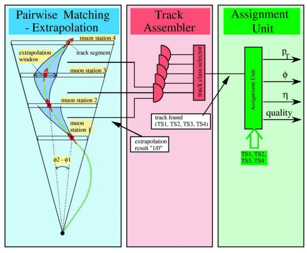
Track-finder electronics is mounted off detector and is implemented using FPGAs
