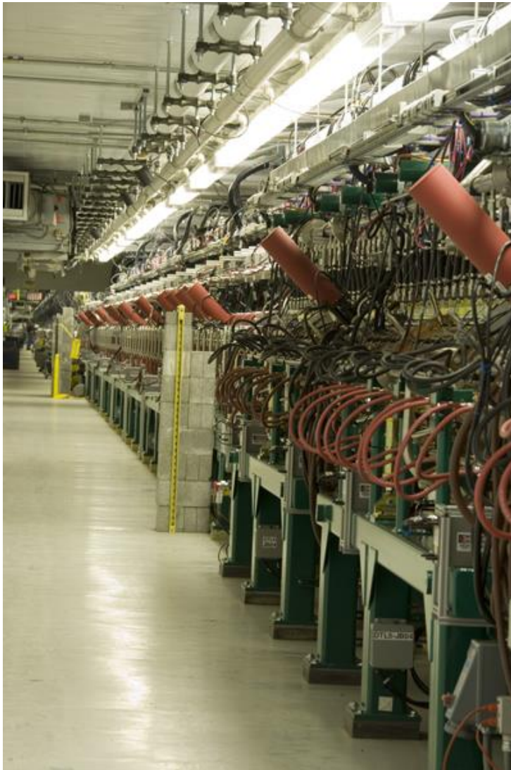
Top; CERN Linac2 Drift Tube Linac: 1978, 202.5 MHz, 3 tanks, final energy 50 MeV, tank diameter 1 meter.
