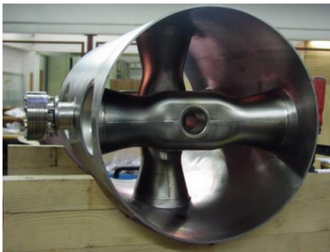
HIPPI Triple-spoke cavity prototype built at FZ Jülich, now under test at IPNO
