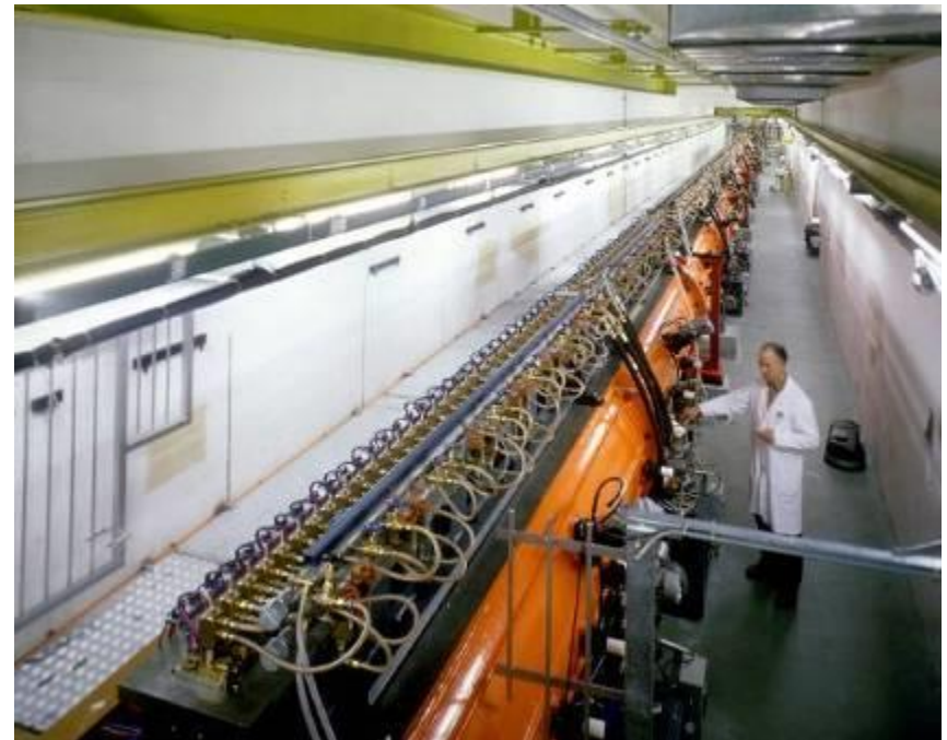
Top; CERN Linac2 Drift Tube Linac: 1978, 202.5 MHz, 3 tanks, final energy 50 MeV, tank diameter 1 meter.
