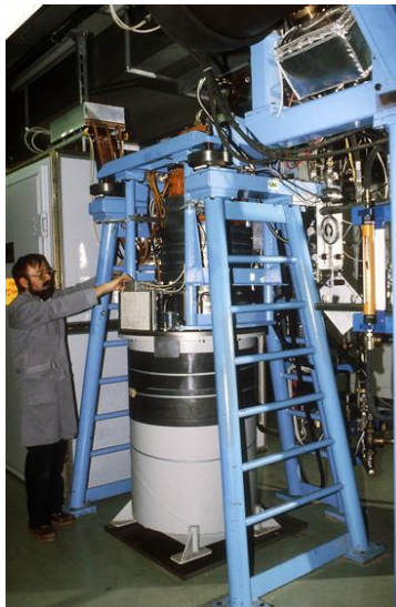
The CERN LIL klystron (3 GHz)
